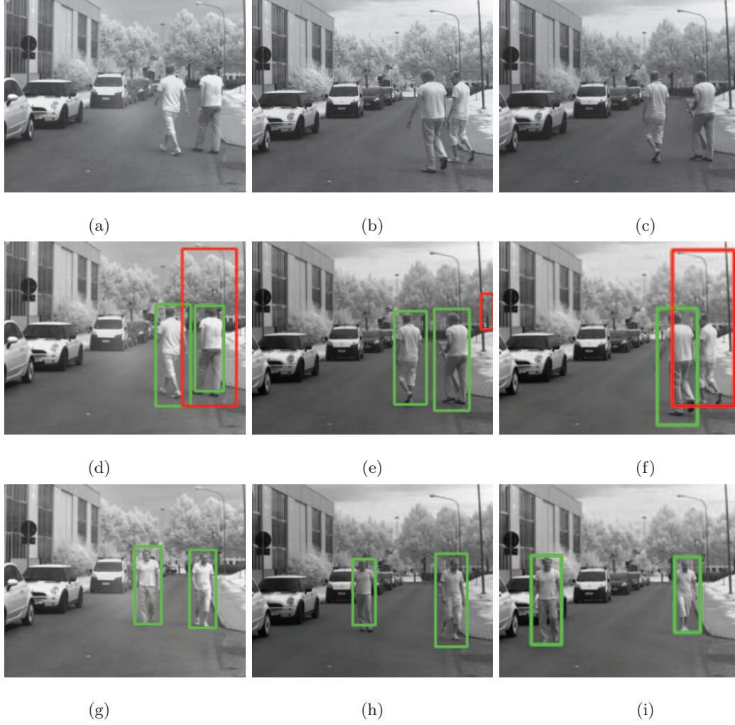
Figure 3.7: Image examples from the sequences showing similar scenes and corresponding output results given by the grammar models: C filter range (a), (d), (g), F2 filter range (b), (e), (h) and F1 filter range (c), (f), (i). False positives produced by the algorithm are surrounded by red BB while true positives are in green BB.
